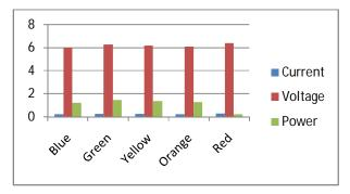
Figure 2: The voltages, current and power variation of the module with different colours of the wavelength of light
