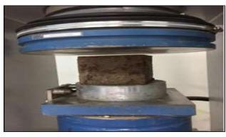
Figure 7: Compression test for the soil sample
