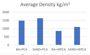
Figure 8: Density of treated soil
