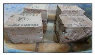
Figure 6: Setup of experiment for porosity test
