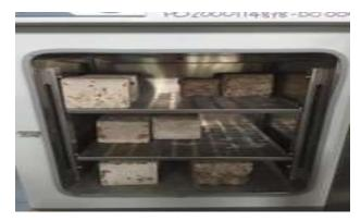
Figure 5: Soil sample placed in the oven
