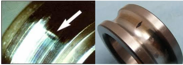
Fig 6: Dentation marks over bearings
