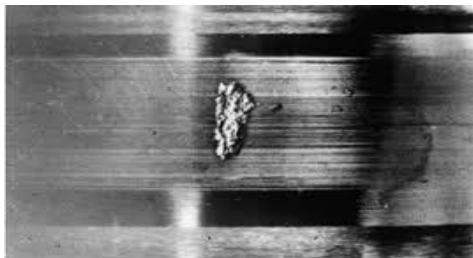
Fig 7: Material deposition on bearing outer race due to fatigue
