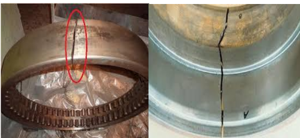
Fig 2: Images of bearings with thermal cracks
