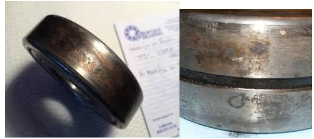
Fig 3: Fretting corrosion in bearings
