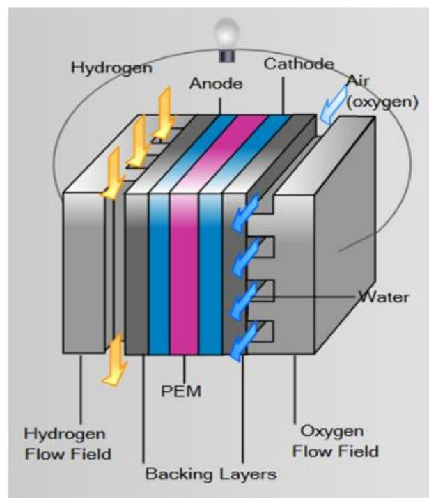
Figure 4: Fuel Cell Cross-Sectional Description
