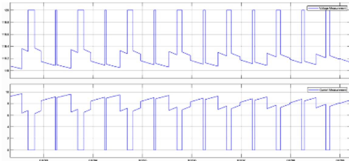
Figure 18: Voltage and Current output of the DC-bus with inverter load connected in standalone simulation.
