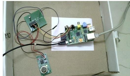
Fig. 5: Sensors connected to GPIO
