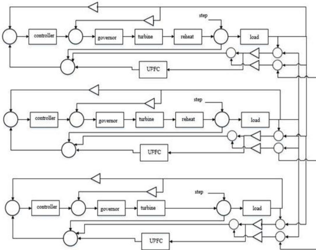
Figure.1: A Three area power system represented by its lock diagram
