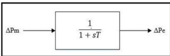
Figure. 2: Model of the Generator
