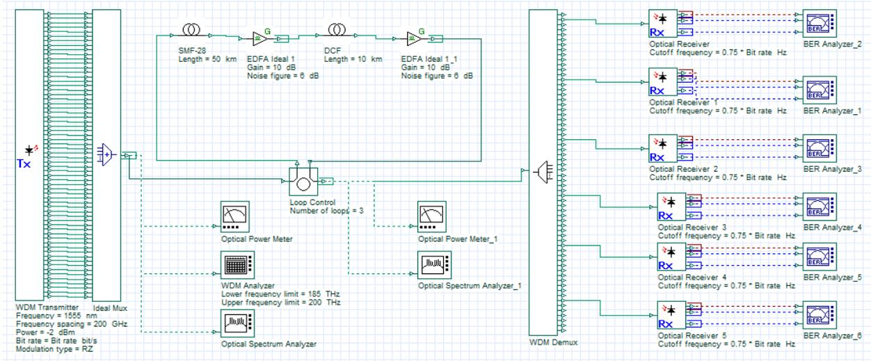
Fig. 1: Schematic Design for 64 Channel DWDM
