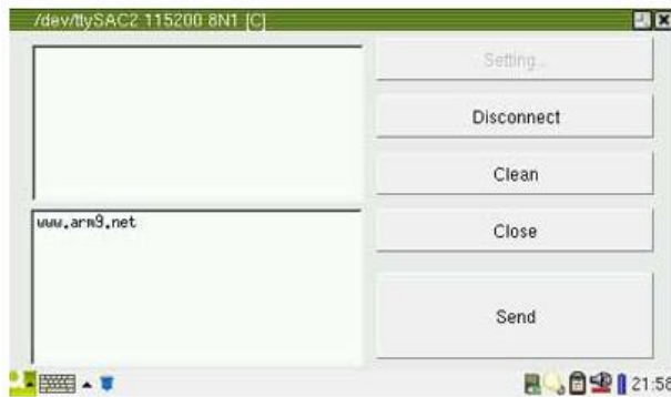
Fig 2: Serial port communication between ARM processor and pc
