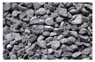
Figure 3: Coarse Aggregate
