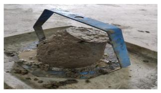
Figure 5: Slump Cone Test
