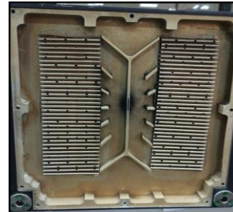
Figure 5: Housing of WMMC LRU with Black Soot
