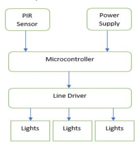
Figure 2: Illustrates the block diagram of street light modules that increase or decrease the intensity of street light using a PIR sensor
