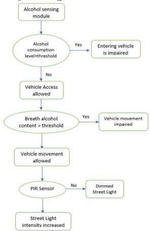
Figure 1: Illustrates the flow chart of the complete module of the light intensity sensor with an alcohol detector
