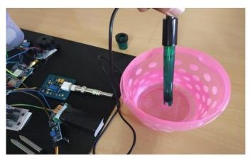
Fig. 4: Snapshot for pH sensor experiment
