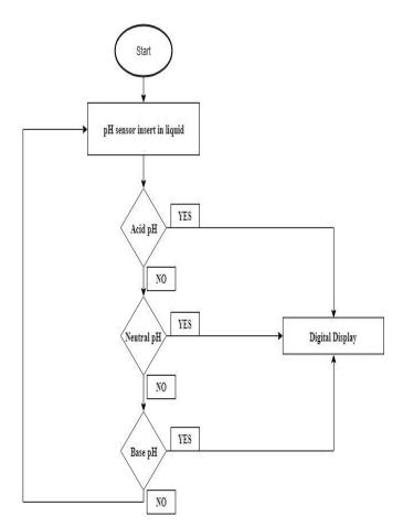
Fig. 5: Control logic for pH sensor
