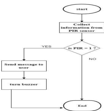
Fig. 6: Control logic for PIR sensor
