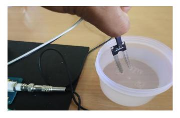
Fig. 3: Snapshot for Level sensor experiment
