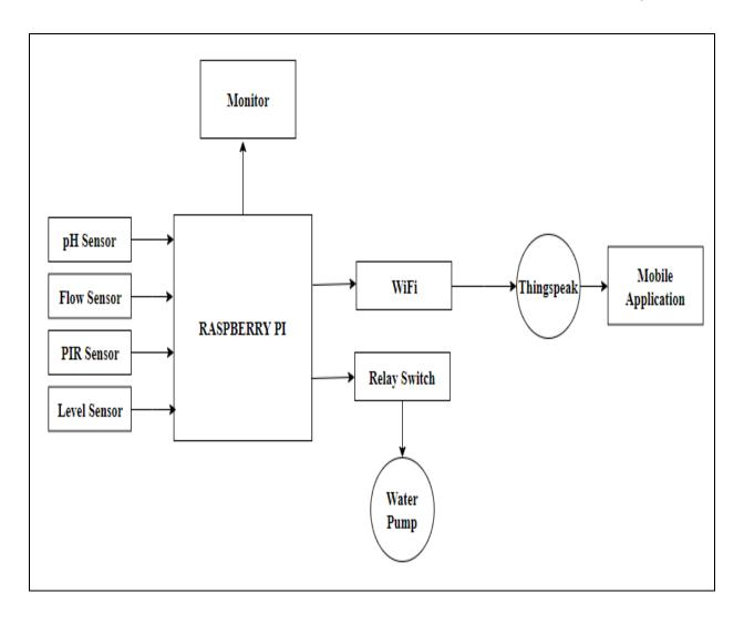
Fig. 1: Block diagram of controller system
