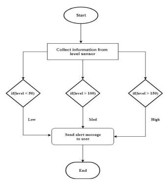
Fig. 2: Control logic for level sensor
