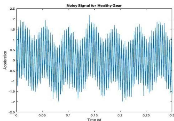
Fig 7: Noisy Signal for Healthy Gear
