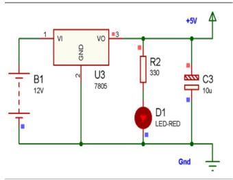
Figure 9 Battery operated +5V power supply
