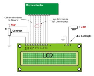
Figure 8 LCD Basic Connection
