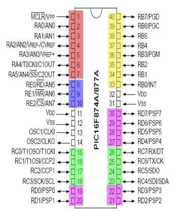
Figure 7 PIC 16F877A Pin Configuration
