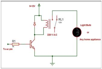
Figure 10 Relays switch board interfacing with the microcontroller
