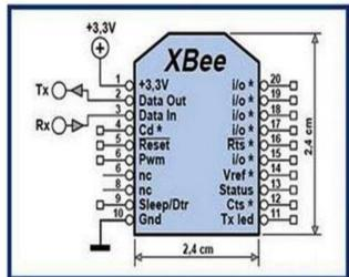
Figure 6 Zigbee pin configuration
