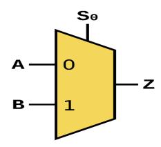
Figure 2: Block diagram of 2:1 multiplexer
