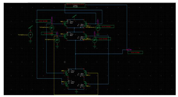
Figure 3: 2:1 Multiplexer using CMOS
