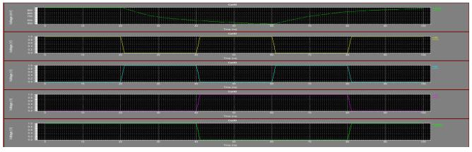
Figure 20: 2:1 Multiplexer output waveform for 45nm
