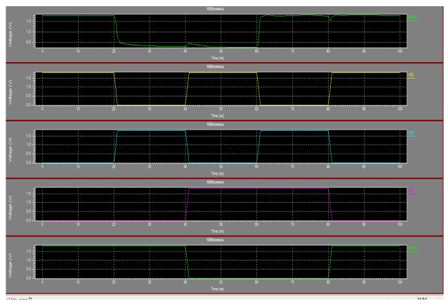
Figure 9: 2:1 Multiplexer output waveform for 180nm
