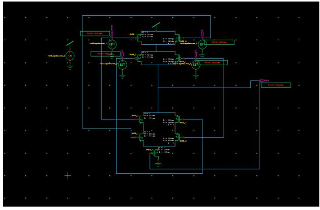
Fig.12: 2:1 Multiplexer using LCpmos technique
