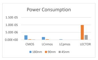
Figure 21: Comparison of power reduction techniques
