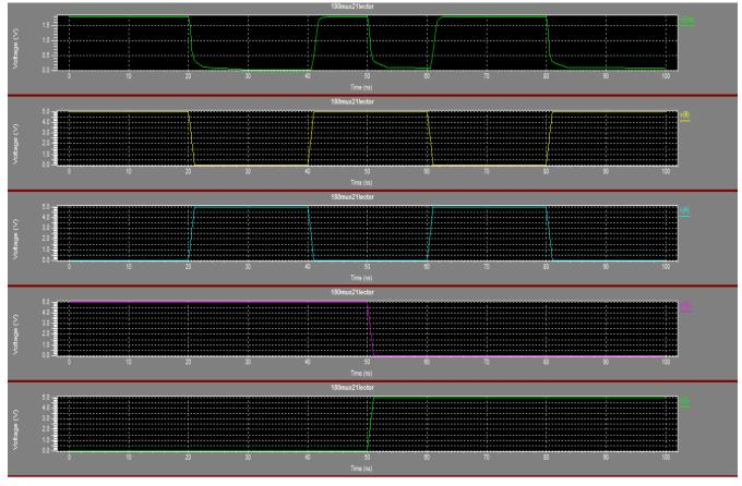
Figure 18: 2:1 Multiplexer output waveform for 180nm
