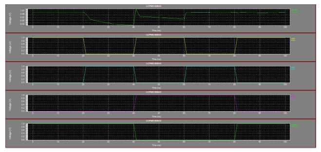
Figure 14: 2:1 Multiplexer output waveform for 90nm
