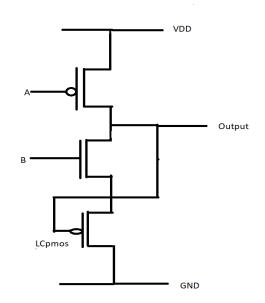
Figure 10: CMOS inverter using L Cpmos
