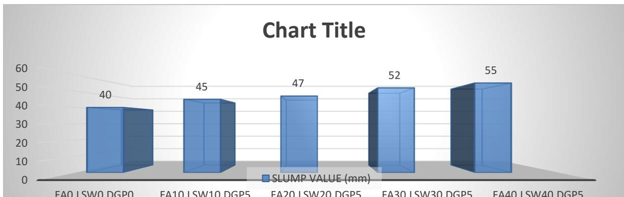
Figure 6: Chart of Slump test
