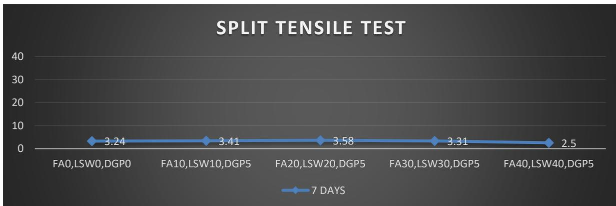
Figure 3: Split tensile test after 7 days
