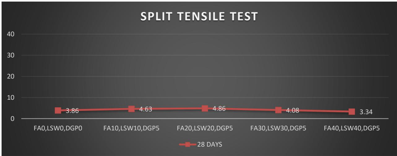
Figure 4: Split tensile test after 28 days
