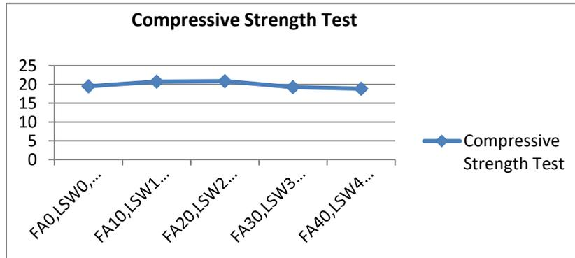
Figure 1: Representation of compressive strength after 7 days
