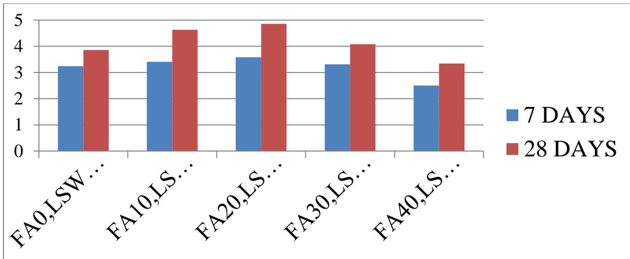
Figure 5: Split tensile test after 7 and 28 days respectively
