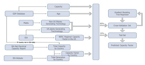
Figure 3: Gas-Fired Power Plant Generation Estimation Workflow
