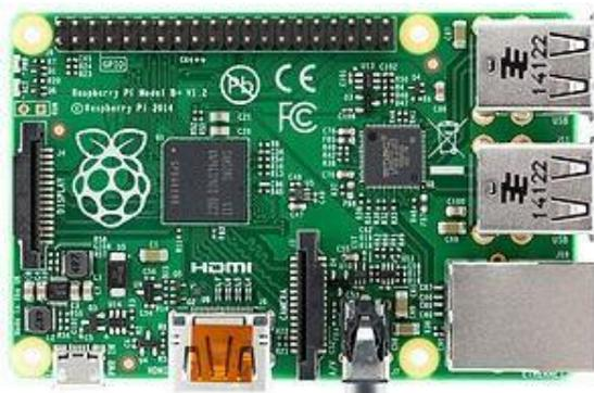
Fig 2: Architecture of Raspberry pi[2]
