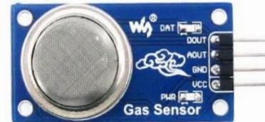
Fig. 5: MQ-7 Gas Sensor
